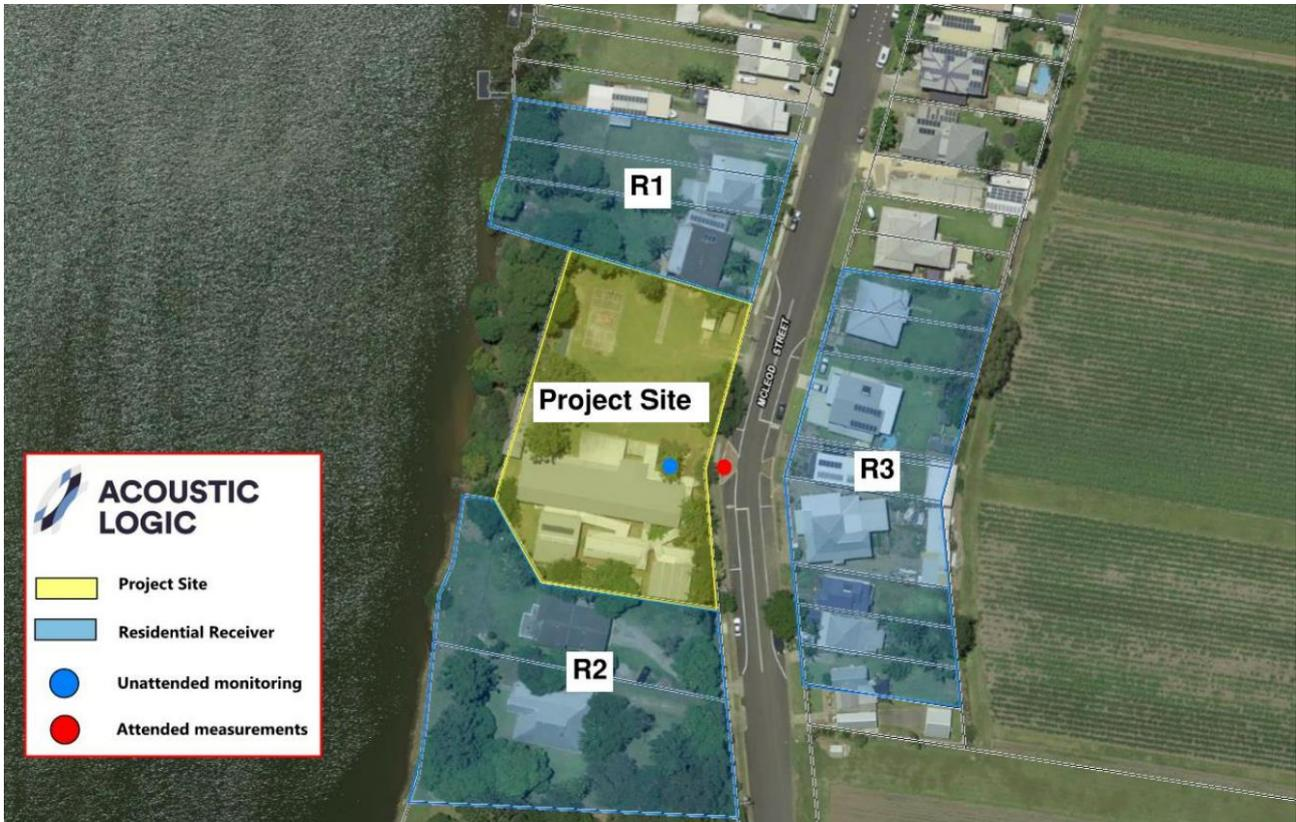
**Figure 34: Location of noise sensitive receivers and monitors (Source: Acoustic Logic)**
